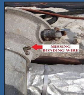
Pneumatic blowers recovered onboard a tank barge explosion had either missing or improperly maintained bonding wires
